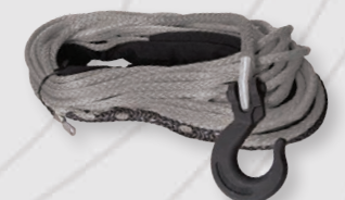
Synthetic Rope 19-52038-100C * 3/8" X 92' Gray Rope Assembly (16,200 lbs. Min Break Force) 19-52516-100C * 5/16" X 92' Gray Rope Assembly (11,700 lbs. Min Break Force) 19-52014-50 1/4" X 50' Gray Rope Assembly (7,740 lbs. Min Break Force) 19-52316-50 3/16" X 50' Orange Rope Assembly (5,440 lbs. Min Break Force)
